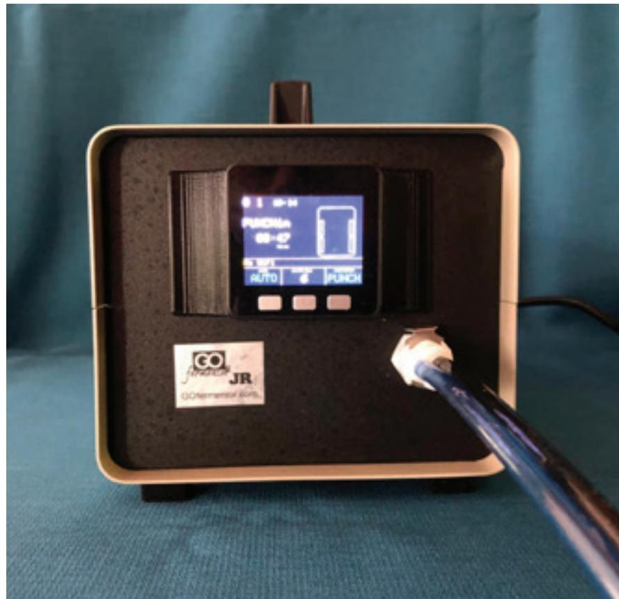
**FIGURE 6:** The controller is set up and monitored by the buttons on the front, where the cycles of punch and press are made. The controller can also be managed by smartphone apps.
