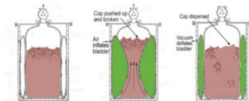
**FIGURE 7:** The punch cycle forces the wine up through the cap into the top of the barrel. Relaxing the bladder pressure lets the juice fall back into the barrel. This sequence is controlled by the remote controller.
