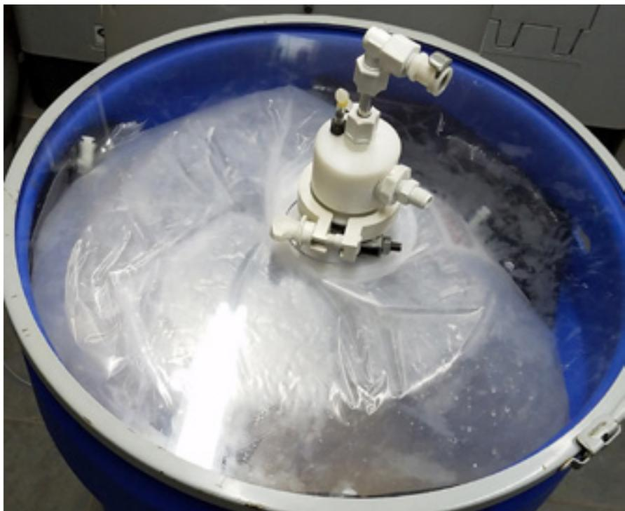
**FIGURE 5:** Here the bag has been secured in the barrel with the barrel lid clamp. The pressure relief valve has been installed, and the sampling port on the top is available for monitoring the fermentation. Removal of the tri-clamp allows the return of sampled juice and the addition of nutrients/malolactic culture during fermentation.
