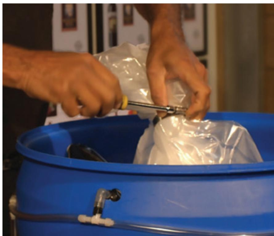
**FIGURE 4:** Once fruit has been added, the slit is folded over and sealed with tape. The bag is then twisted into a tight roll and clamp-fitted around the roll. Heavy duty tape is then wrapped around the clamp to prevent damage to the bag while in the barrel.
