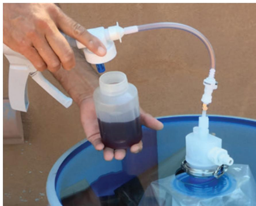
**FIGURE 8:** Sampling of wine is done through this vacuum pump that brings wine up through the sample tube into the 250 ml bottle. After sampling, the wine can be returned to the barrel by removing the tri-clamp and then reseating it onto the port.
