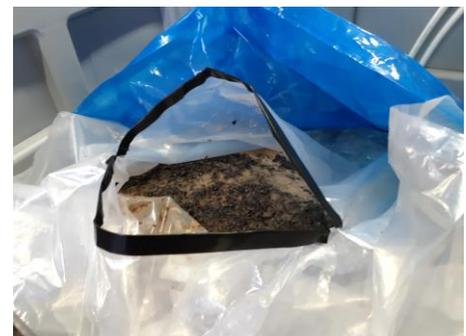
3. Apply tape along the length of the cut on both sides and fold over the edges. This will help hold the cut open and also help during closing the liner after filling.
