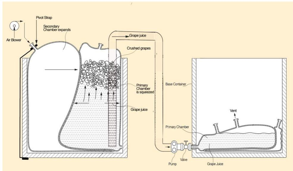
7. Start the wine transfer pump to transfer the free-run juice. At first, the pump will simply remove the headspace gas and you should see the headspace collapsing. The juice will start to flow once all the gas is removed.
