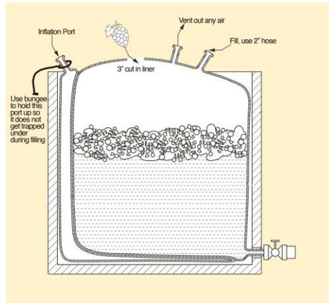
2. Placement of the cut is crucial and should be made inside the triangle formed by seams between the vent port and the inflation chamber, making sure not to cut into any of the welded seams of the liner. We recommend a cut no longer than 24 inches
