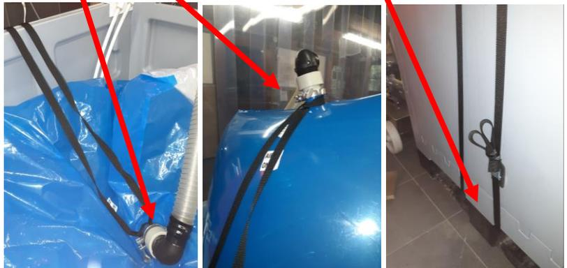
**Note:** During punching operations the slack may not be taken up completely but the PIVOT STRAP is **essential** during pressing to hold the air chamber vertical and in position.
