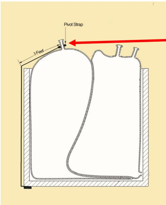
Double loop and/or knot PIVOT STRAP around blue inflation port to prevent from slipping off
