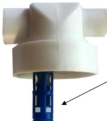
The valve is in this cage. If it is stuck up then the sampler will not pump. Shake it so it moves freely up and down and stays in the down position.
