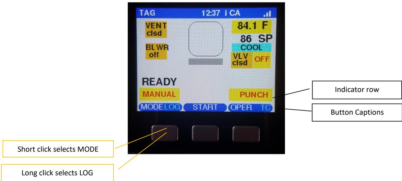
The GOfermentor panel has just three buttons. If a button has only one function, then the caption is printed in the center of the button. If the button has two functions, then both are printed on the caption – the function on the left is printed in white and corresponds to a short click. The caption on the right is printed in cyan and is activated by a long click. Each button can have up to 2 functions.
