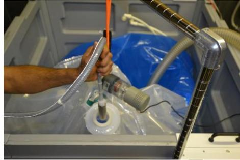
2. Use the supplied TriClamp to secure the sampler/temperature probe.
