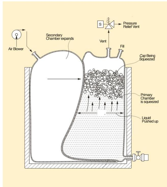
Punch of the cap may be initiated at any time in the fermentation. It can also be performed after initial *must* adjustment to mix nutrient additions if desired.
