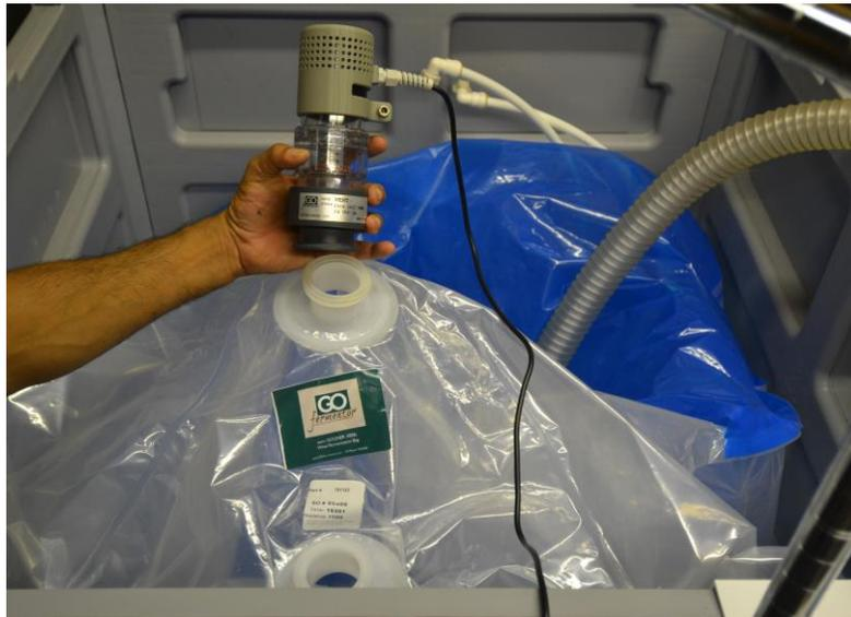
6. Use the supplied suspension cord to hang the VENT VALVE from the support pole located on the left side of the GOFERMENTOR control panel. This keeps the VENT assembly from falling into the GOBASE. Adjust the cord so that the VENT assembly is above the lip of the outer container.
