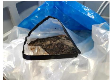
3. Apply tape along the length of the cut on both sides and fold over the edges. This will help hold the cut open and also help during closing the liner after filling.
