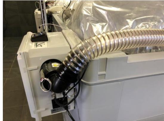
9. Power up the control panel. Once the MAIN CONTROL window is displayed press the PUNCH button and verify that the VENT valve opens. You will hear a click and you can see the valve open about ½” through the clear VENT valve assembly. Press the flashing CANCEL button and verify that the valve closes. The VENT assembly is actuated electrically during PUNCH operations. It also has a spring-loaded pressure relief valve that automatically vents if the GOLINER pressurizes beyond safety limits.
