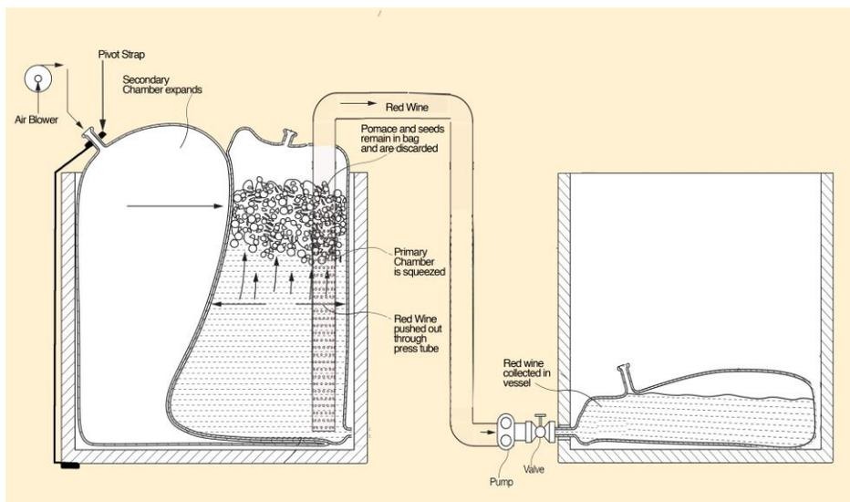
7. Start the wine transfer pump to transfer the free-run wine. At first, the pump will simply remove the head space gas and you should see the headspace collapsing. If you do not observe the headspace being removed, there is an air leak into the headspace or the pump is insufficient. **You must resolve this otherwise the pressing operation is not possible.** The wine will start to flow once all the gas is removed. Avoid pumping too fast as this will draw in the cap.
