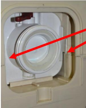
Make sure tabs are locked into the grooves on both sides!
