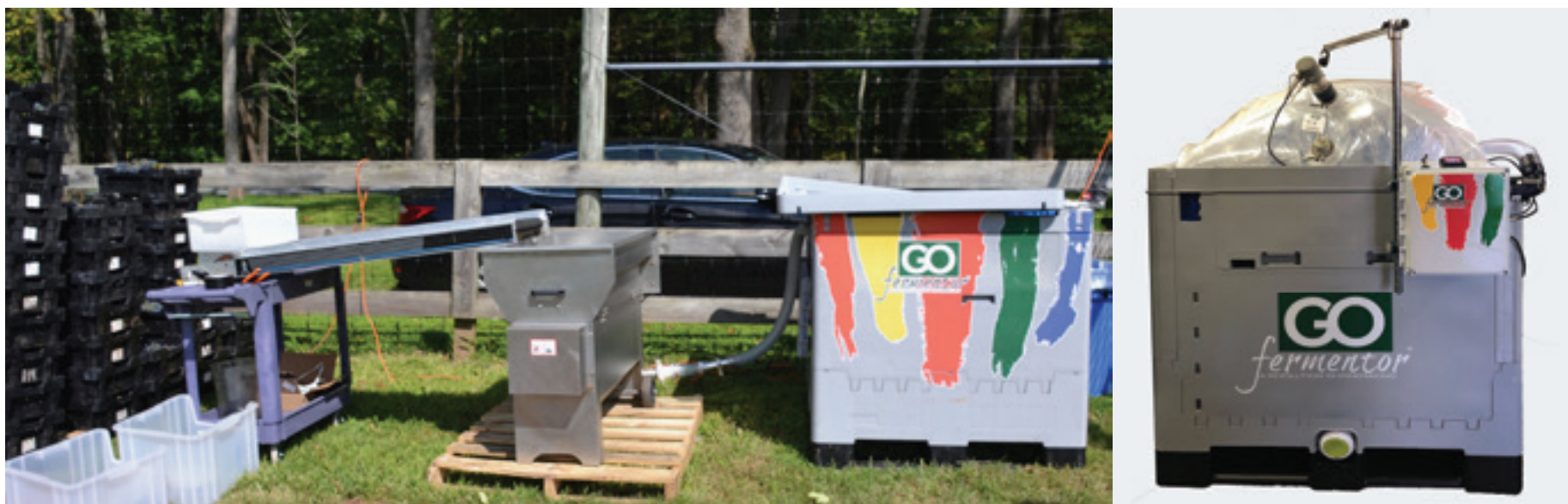
FIGURE 1 (RIGHT) The grapes go from the crusher to a macrobin containing GOfermentor bags. (LEFT) The GOLiner inflates in the macrobin.
