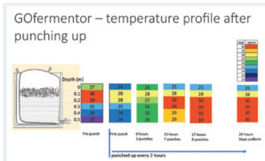
**FIGURE 10B** GOfermentor’s ability to mix the juice and the skins more times a day and over many more days than is usually possible for most wineries to do, results in a warmer average temperature for red wines. This seems to be a primary reason for the better extraction of fruit flavors in wine that has been fermented in this way.
