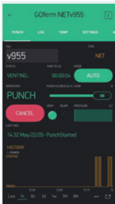
FIGURE 4 Managing GOfermentor functions is easier with the GOfermentor App that allows the user to enter information directly to the controller.
